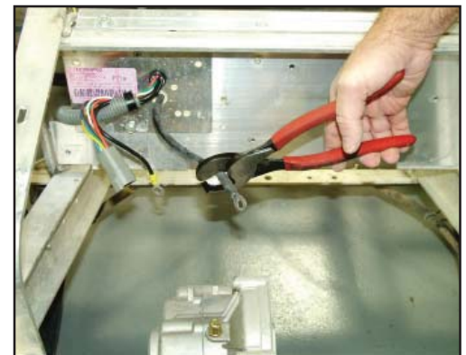
7. Remove Battery Negative
