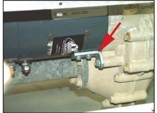
10. Install Motor Clip
