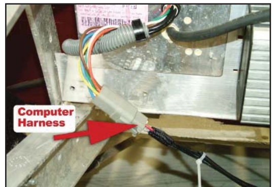
18. Install Computer Harness & Black Jumper
